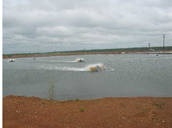
Aquaculture ponds are aerated to maintain the Biological Oxygen Demand (BOD) levels
